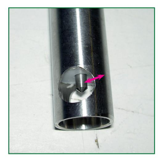
When the probe comes into contact with water electricity is conducted between the metal point in the centre of the probe and the outside of the probe sending a signal to the meter giving the 'water' tone and visual alarm.
