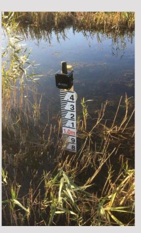
Dip meters are your friend: Water level loggers and sensors are very accurate, they are field robust, have great long term stability and are available at a relatively low cost. Nonetheless, despite their accuracy and long term stability it is necessary to verify that they are performing to specifications. This is done with a dip meter.
