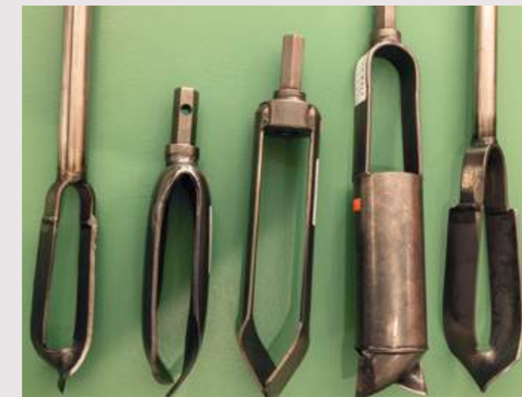
Different hand auger heads to cope with different soils
