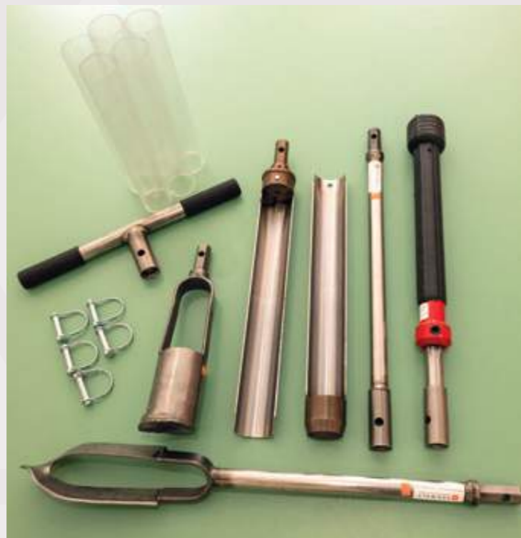
Split tube sampler
