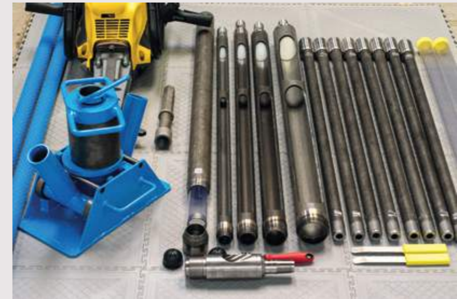
Typical window sampling set to 8 metres
