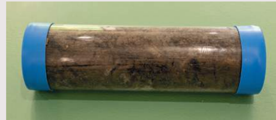
Semi-disturbed sample captured within a liner
