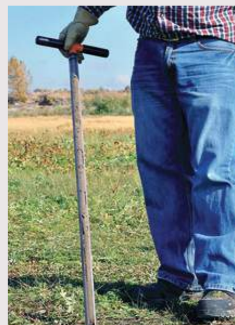
Filled 100cm gouge auger
