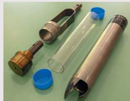
Liner sampler within a standard hand auger
